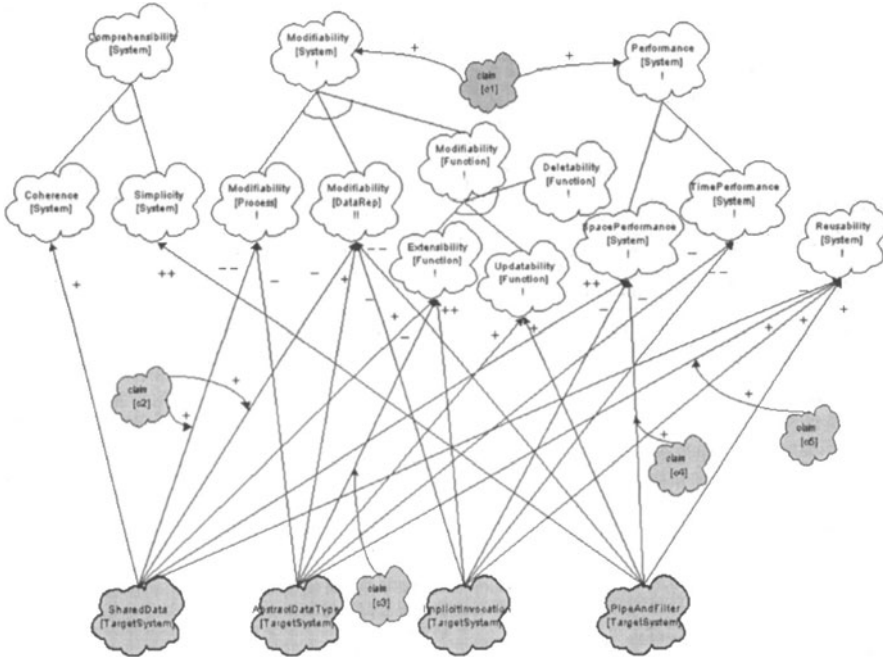
Figure 8b. A model that assesses architectural choices within software. Options within the model are the leaf nodes shown in gray. These options can be architectural decisions such as the use of abstract data types, implicit invocation, pipe & filter methods, or shared data. Some links in the model are dependant of various claims c_1, \dots, c_5 shown in Fig 8a. For example, claim[c2] is Parnas's [42] argument that having a single share data model across an entire application has a negative impact on the modifiability of that process. The inference rules of this diagram are shown in Fig 8c.
